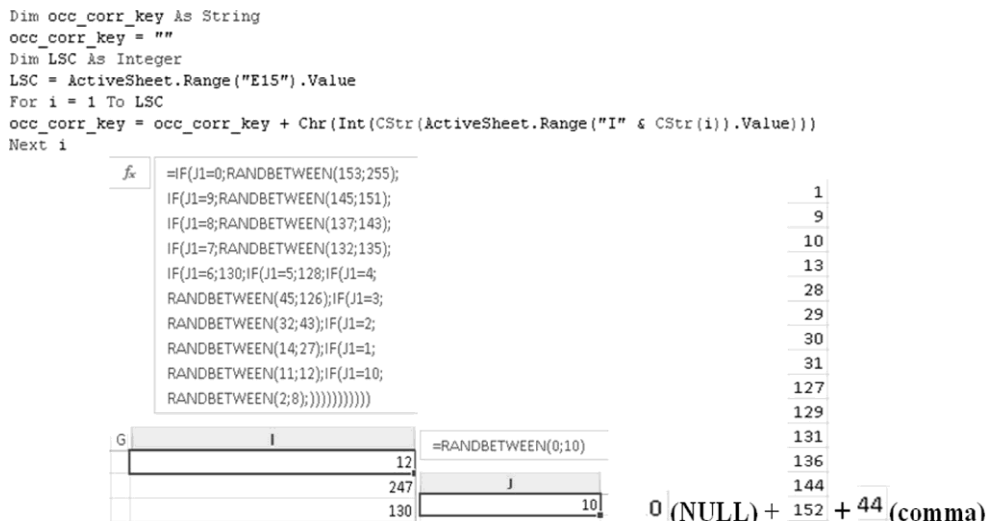
Figure 6. ASCII codes of characters to avoid in 64B3AC's substitutions (VBA exceptions / errors)
